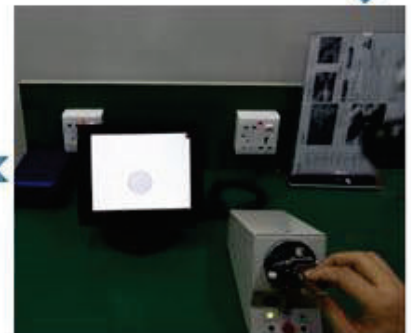
Cleaning end face
