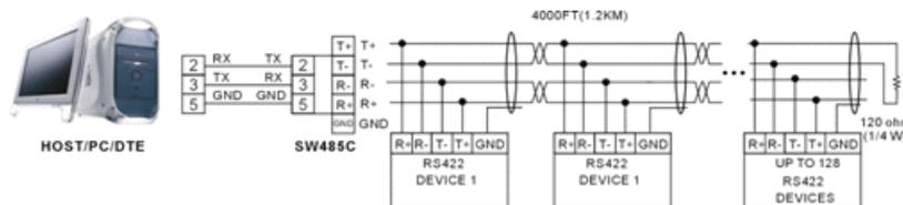
Figure 4: Master/Slave multi-drop configuration in RS422 mode
