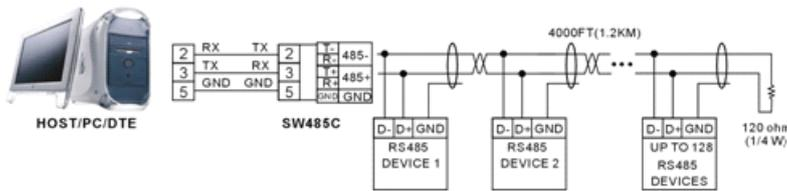
Figure 2: Master/Slave multi-drop configuration in RS485 mode
