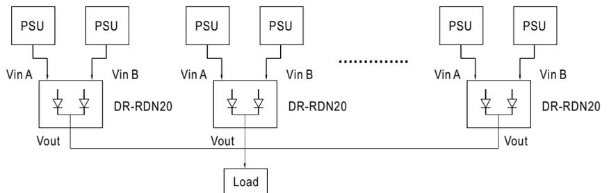
**3. Single Use: Connecting only one PSU to one DR-RDN20 to reduce the stress of the diodes and hence increase the reliability**
