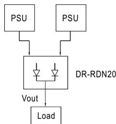
**2. 1+N Redundancy: Using more PSUs as the redundant units to increase the reliability**
