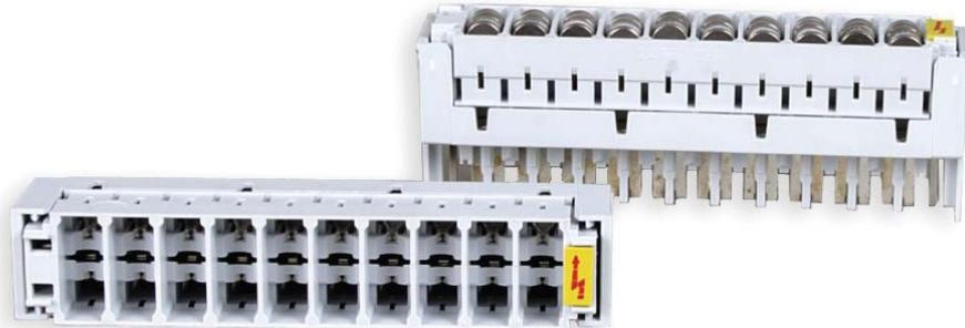
LSA-PLUS® Protection Magazine 2/10, houses 10 nos 3 pole GD Tube or Overvoltage arrestors. The magazine is plugged on disconnection module 10 pairs to provide overvoltage protection to connected lines.
