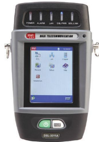
DSL-3011A xDSL Tester is a handheld ADSL/ADSL2/ADSL2+ line test and analysis instrument, which can test physical layer, network layer and application layer quickly and accurately. It is a necessary tool for xDSL line deployment and maintenance. This product applies to deployment and maintenance of operators's broadband service.
