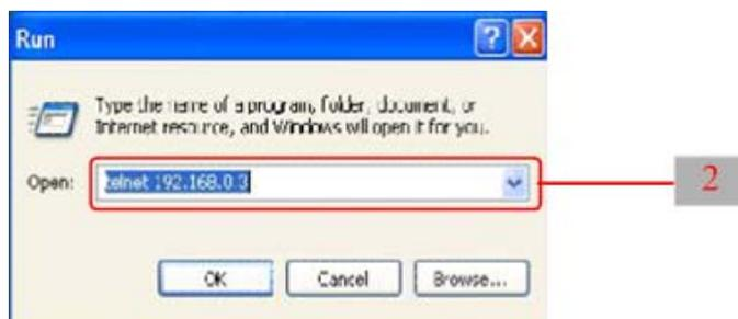
2. Click “OK”, setting the IP of device by telnet. Choose the menu by ↑↓←→ of the keyboard and quit by “ESC” key.
