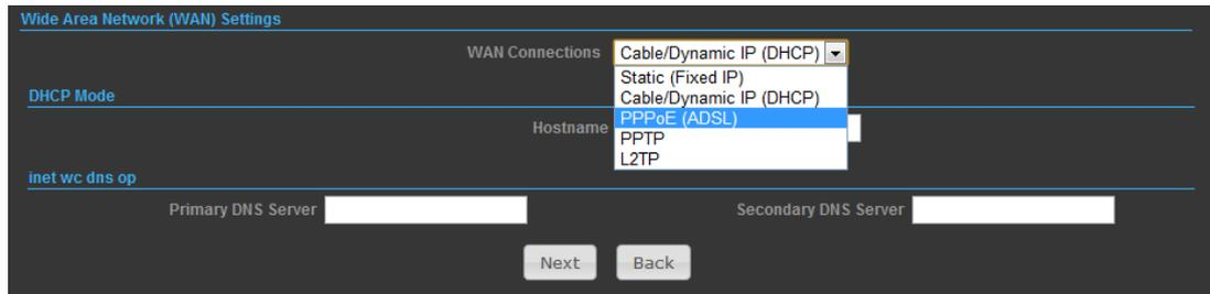
The screenshot shows the 'Wide Area Network (WAN) Settings' screen. The 'WAN Connections' dropdown menu is open, showing options: Cable/Dynamic IP (DHCP), Static (Fixed IP), Cable/Dynamic IP (DHCP), PPPoE (ADSL) (highlighted), PPTP, and L2TP. Below the menu, there are fields for 'DHCP Mode', 'Hostname', 'Primary DNS Server', and 'Secondary DNS Server'. 'Next' and 'Back' buttons are at the bottom.
