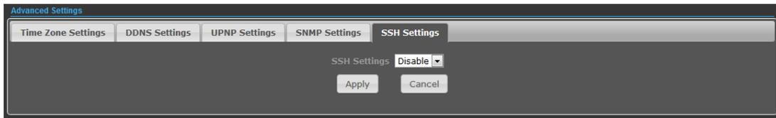
**SSH Settings** – Secure Shell. Enable your AP unit to access secure shell (SSH) based network device. Default setting is Disabled.
