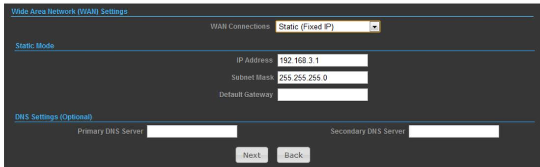
The screenshot shows the 'Wide Area Network (WAN) Settings' interface with 'Static Mode' selected. The 'WAN Connections' dropdown is set to 'Static (Fixed IP)'. Fields for 'IP Address' (192.168.3.1), 'Subnet Mask' (255.255.255.0), and 'Default Gateway' are visible. There are also fields for 'Primary DNS Server' and 'Secondary DNS Server'. 'Next' and 'Back' buttons are at the bottom.
