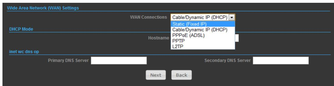
The screenshot shows the 'Wide Area Network (WAN) Settings' interface. The 'WAN Connections' dropdown menu is open, displaying options: Cable/Dynamic IP (DHCP), Static (Fixed IP) (highlighted), Cable/Dynamic IP (DHCP), PPPoE (ADSL), PPTP, and L2TP. Below the menu, there are fields for 'DHCP Mode', 'Hostname', 'Primary DNS Server', and 'Secondary DNS Server'. 'Next' and 'Back' buttons are at the bottom.
