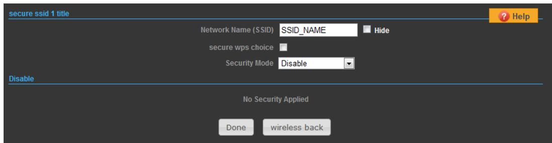
The screenshot shows the 'Security Setup' screen. It includes: 'Network Name (SSID)' (SSID\_NAME) with a 'Hide' checkbox, 'secure wps choice' (disabled), and 'Security Mode' (Disable). A 'Disable' link is visible. At the bottom, it says 'No Security Applied' and has 'Done' and 'wireless back' buttons.
