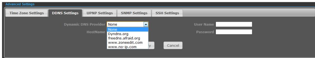
**DDNS Settings** — DDNS lets you assign a fixed host and domain name to dynamic Internet IP address. It is useful when you are hosting your own website, FTP server, or other server behind the AP. Before using this feature, you need to sign up for DDNS service at [www.dyndns.org](http://www.dyndns.org), a DDNS service provider.
